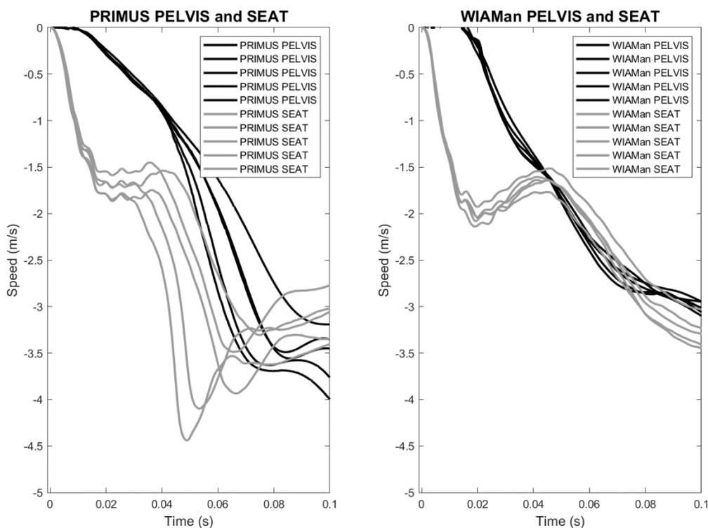
**Figure 18 Comparisons Pelvis (black) and Seat (gray) Speeds (150g tests)**
