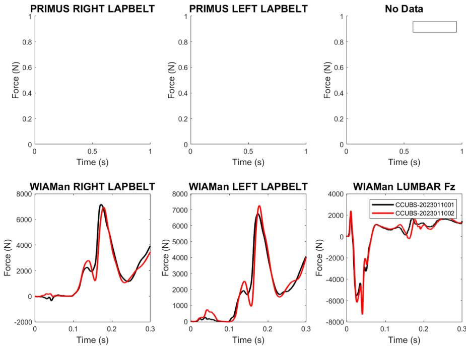
Figure 8 SAE Channel Class CFC60 Lapbelt Loads and CFC600 HIII Lumbar Vertical Load (350g)
