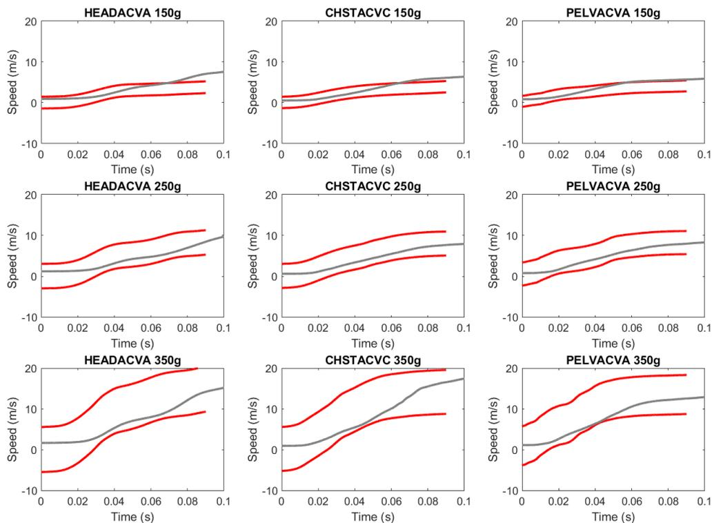
**Figure 19 Average Body Segment Resultant Speed (PRIMUS) versus Speed Corridors (WIAMan)**
