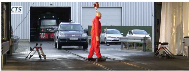
Figure 9: The test setup, where a biofidelic and a NAMI-dummy under identical conditions are impacted with a VW Touareg
