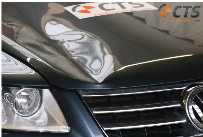
Figures 14-16: Vehicle damages to the VW Touareg
