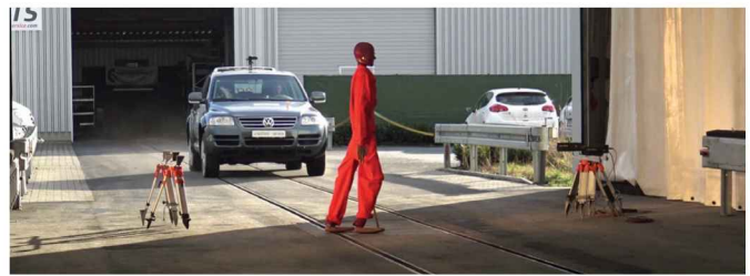
Figure 9: The test setup, where a biofidelic and a NAMI-dummy under identical conditions are impacted with a VW Touareg
