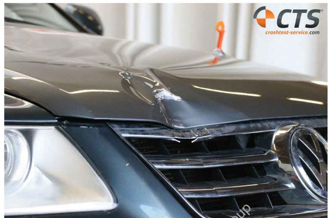
Figures 14-16: Vehicle damages to the VW Touareg
