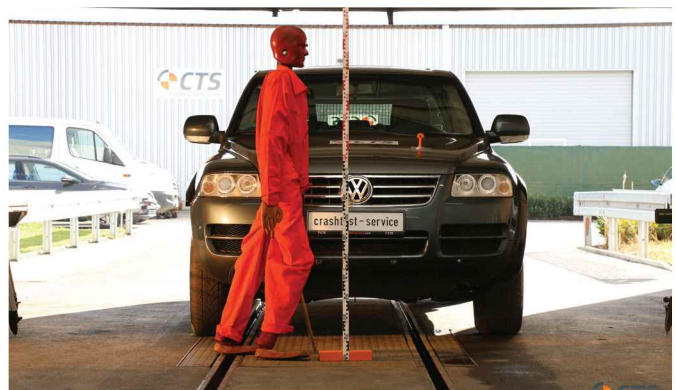
Figure 10: The test setup, where a biofidelic and a NAMI-dummy under identical conditions are impacted with a VW Touareg
