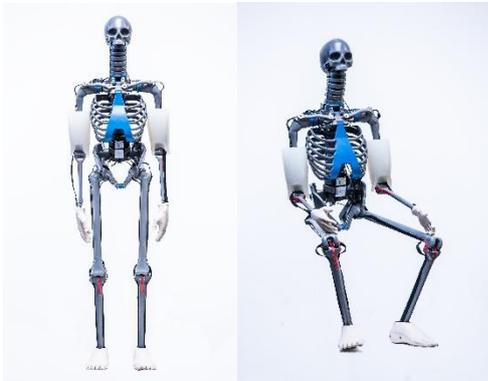
Bone substitute material imitates the mechanical properties of human bones (e.g. breaking strength). Soft tissue replacement material is also similar to human tissue (e.g. hysteresis). Tendons and cruciate ligaments in knee and arm joints correspond to human strength levels.
