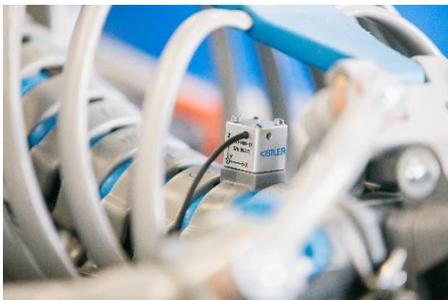
Positions for the in-dummy sensors from Kistler include the head, chest area and hip. A LAN cable allows readout from the data logger positioned in the chest area.
