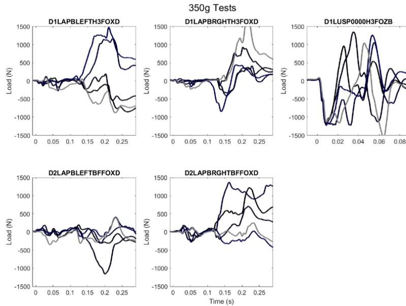
**Figure 9 SAE Channel Class CFC60 Lapbelt Loads and CFC600 HIII Lumbar Vertical Load (350g)**
