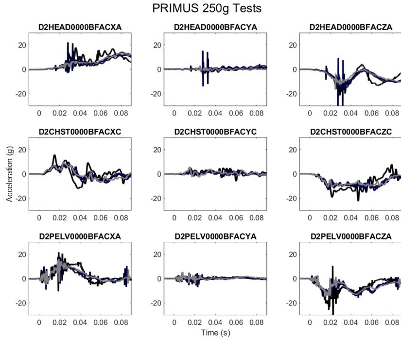
**Figure 13 PRIMUS SAE Channel Class CFC1000 Head, Chest, and Pelvic Accelerations (250g)**
