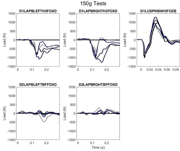
**Figure 7 SAE Channel Class CFC60 Lapbelt Loads and CFC600 HIII Lumbar Vertical Load (150g)**
