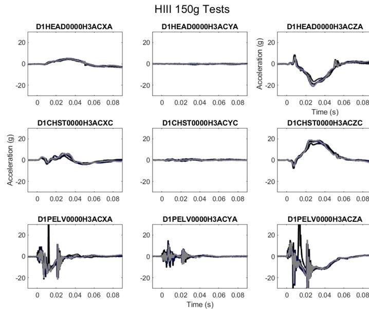
**Figure 10 HIII SAE Channel Class CFC1000 Head, Chest, and Pelvic Accelerations (150g)**
