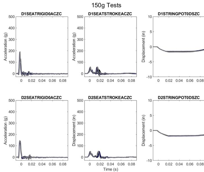
**Figure 4 SAE Channel Class CFC180 Seat Accelerations and Vertical Displacement (150g)**
