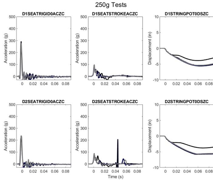
**Figure 5 SAE Channel Class CFC180 Seat Accelerations and Vertical Displacement (250g)**
