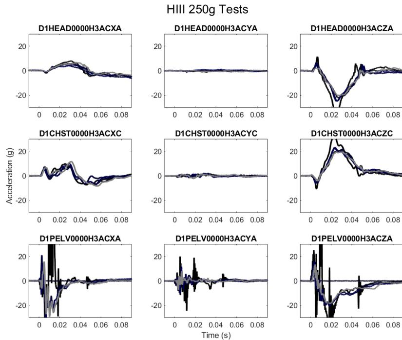
Figure 12 HIII SAE Channel Class CFC1000 Head, Chest, and Pelvic Accelerations (250g)
