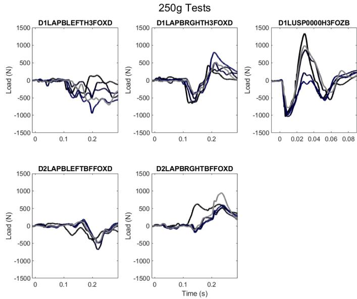
**Figure 8 SAE Channel Class CFC60 Lapbelt Loads and CFC600 HIII Lumbar Vertical Load (250g)**
