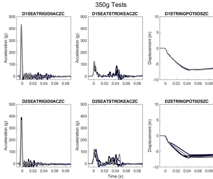
**Figure 6 SAE Channel Class CFC180 Seat Accelerations and Vertical Displacement (350g)**
