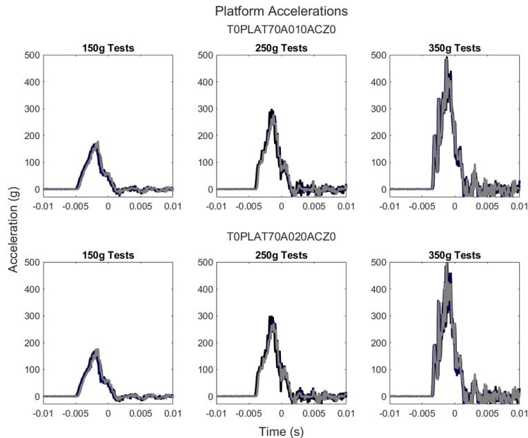
**Figure 2 Unfiltered Input (Platform) Accelerations**
