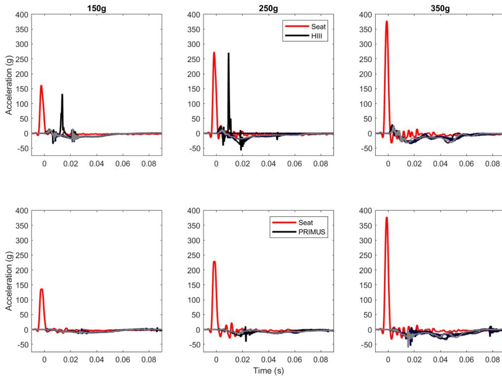
**Figure 17 SAE Channel Class CFC180 Seat Rigid Mount (avg) and SAE Channel Class CFC1000 Pelvic Z Accelerations**
