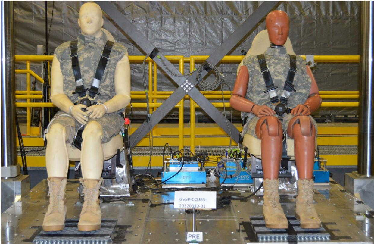
**Figure 1 CCUBS test setup. HIII on the right (Position 1), PRIMUS on the left (Position 2).**
