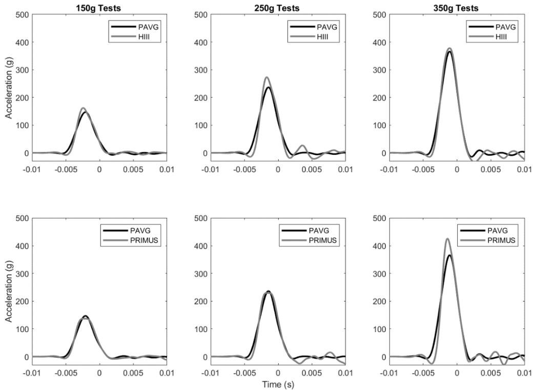
**Figure 16 SAE Channel Class CFC180 Platform (AVG) and SAE Channel Class CFC180 Seat (AVG) Accelerations**
