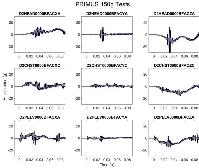
Figure 11 PRIMUS SAE Channel Class CFC1000 Head, Chest, and Pelvic Accelerations (150g)
