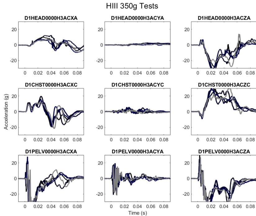
**Figure 14 HIII SAE Channel Class CFC1000 Head, Chest, and Pelvic Accelerations (350g)**
