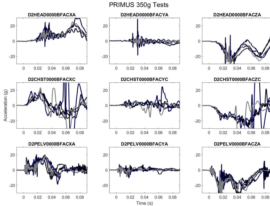
**Figure 15 PRIMUS SAE Channel Class CFC1000 Head, Chest, and Pelvic Accelerations (350g)**
