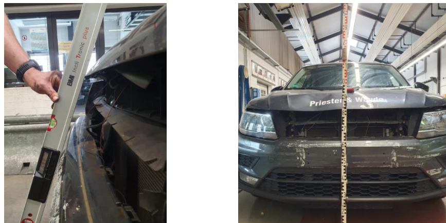
Figure 3. Vehicle measurement and categorization according to IHRA method, example SUV.
