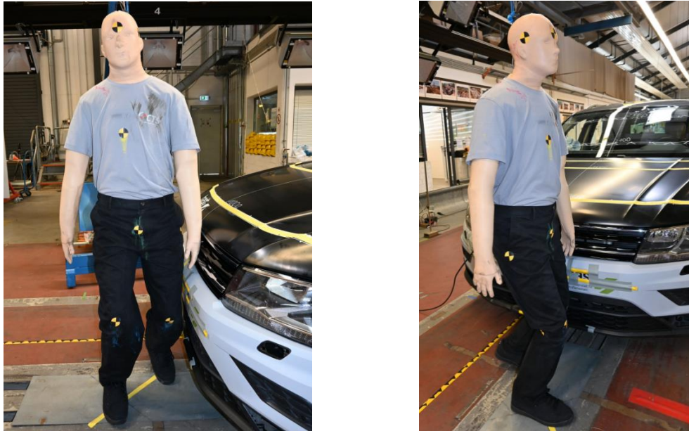
Figure 1. 50th percentile biofidelic dummy „Primus Unbreakable“.
