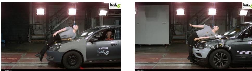
Figure 14. Chest contact at 40 km/h lateral impacts.
