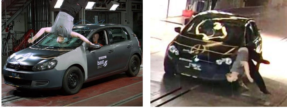
Figure 10. Dummy trajectories during Sedan impact..
