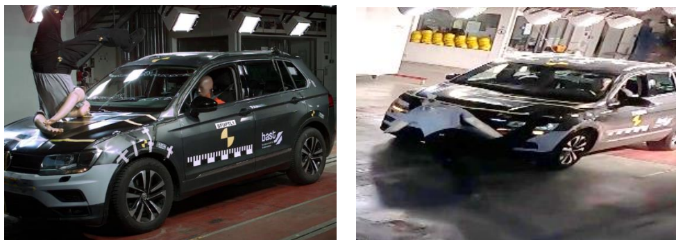
Figure 9. Dummy trajectories during small SUV impact.
