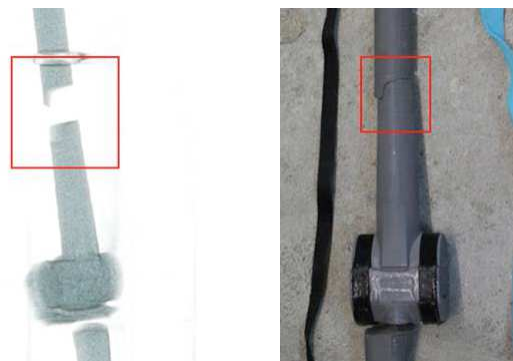
Figure 12: CT scan vs. exposed dummy femur.
