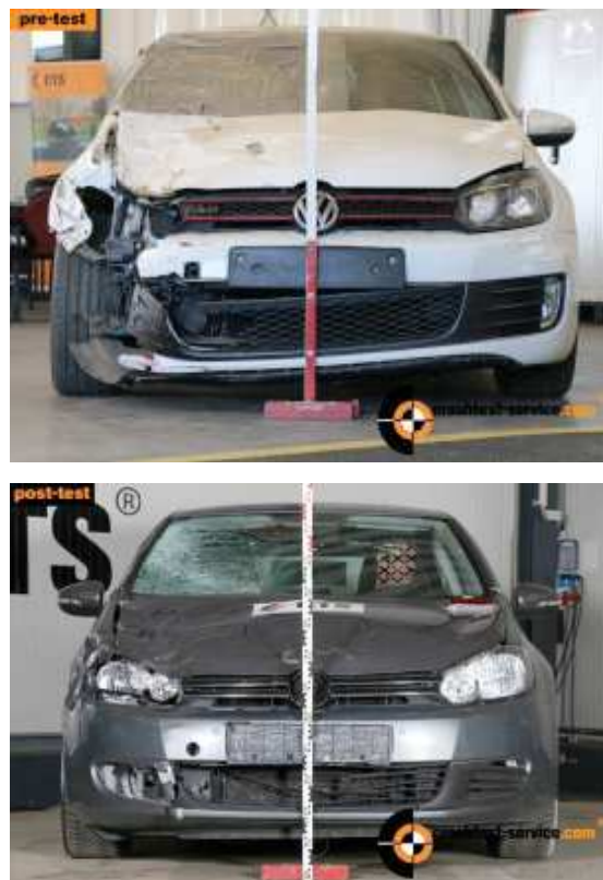
Figure 7: Vehicle damage in the actual accident (upper photo) vs. reconstruction in a crash test (bottom photo) [15].
