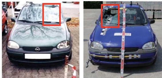
Figure 14: Car damage after the accident (left) [19] and after the crash test (right), speed: 53 km/h.
