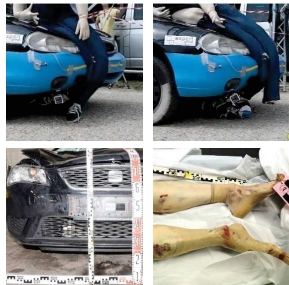
Fig 13: Pull-under-effect with torn-off foot in the test, speed v_k = 71 km/h (above) and partially torn-off foot after real accident (below) [18].
