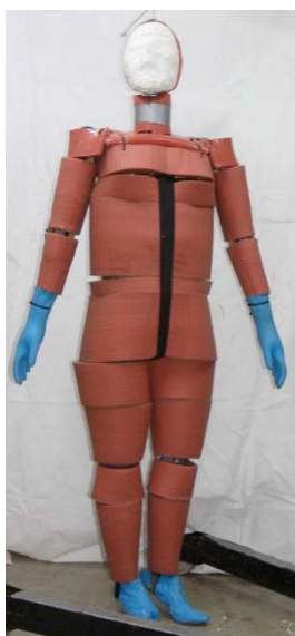
Figure 6: Specific second generation dummy (here depicted without outer cover in order to illustrate the specific component tissue parts of the surrogate for a 163 cm female weighing 80 kg)
