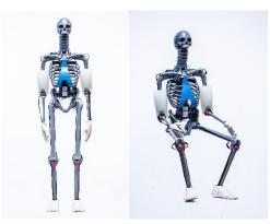
Bone substitute material imitates the mechanical properties of human bones (e.g. breaking strength). Soft tissue replacement material is also similar to human tissue (e.g. hysteresis). Tendons and cruciate ligaments in knee and arm joints correspond to human strength levels.
