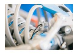
Positions for the in-dummy sensors from Kistler include the head, chest area and hip. A LAN cable allows readout from the data logger positioned in the chest area.
