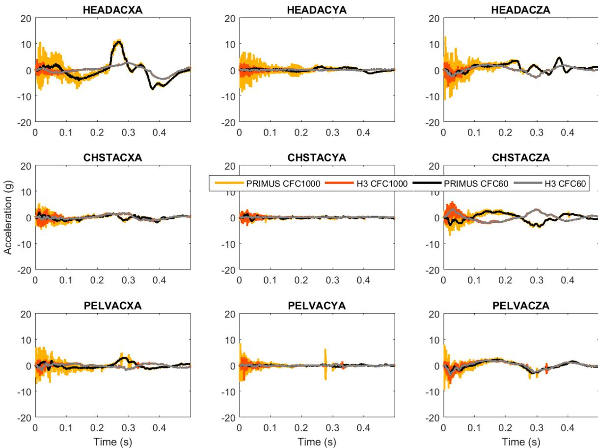
**Figure 10 Comparison of ATD Responses at CFC1000 and CFC60**
