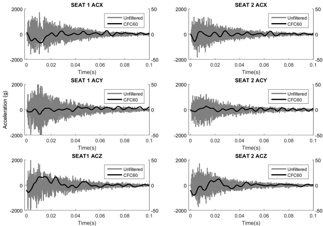
**Figure 8 Seat Accelerations Filtered at CFC60**
