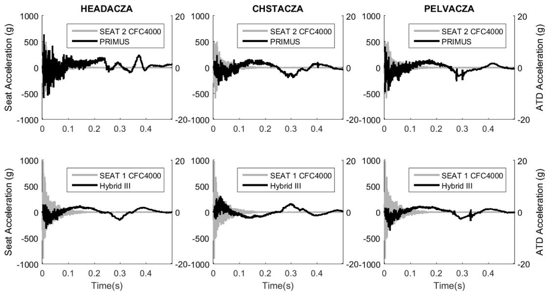
**Figure 9 ATD CFC1000 Responses Compared to Seat CFC4000 Accelerations**
