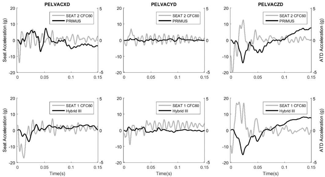
**Figure 3 SAE Channel Class CFC60 ATD Pelvis Responses Compared to SAE Channel Class CFC60 Seat Accelerations**
