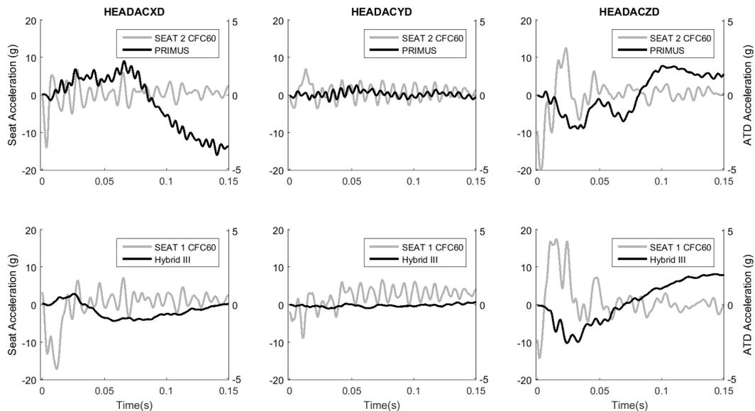
**Figure 1 SAE Channel Class CFC60 ATD Head Responses Compared to SAE Channel Class CFC60 Seat Accelerations**
