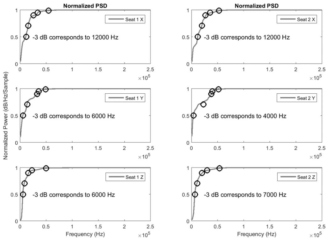
**Figure 4 Integrated Normalized Acceleration Spectral Densities for the Position 1 and 2 seats**
