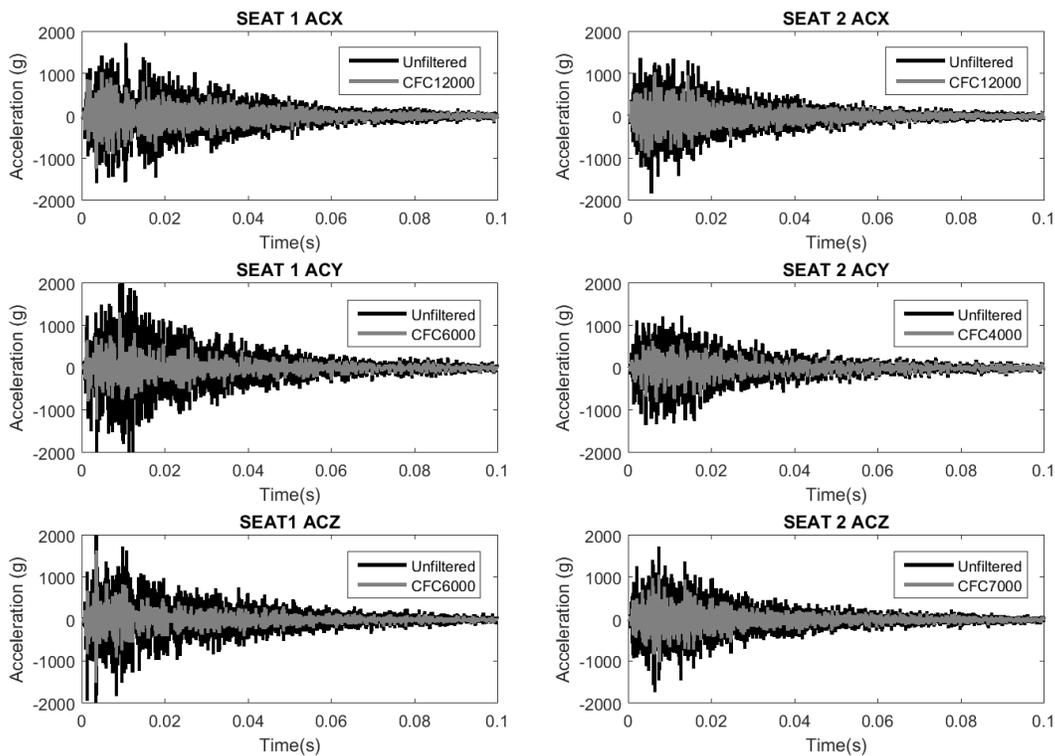
**Figure 5 Seat Acceleration Data Filtered at -3dB Points Identified**
