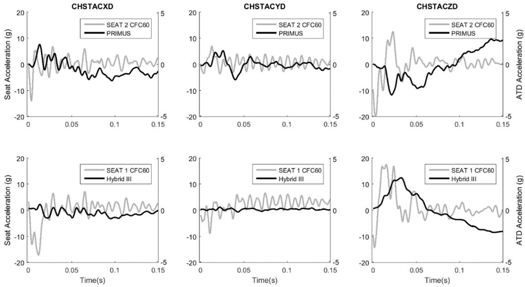
**Figure 2 SAE Channel Class CFC60 ATD Chest Responses Compared to SAE Channel Class CFC60 Seat Accelerations**
