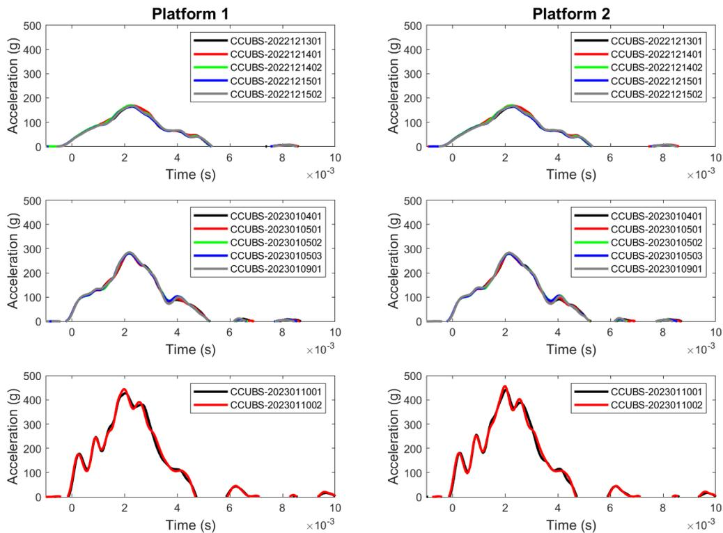
**Figure 2 SAE Channel Class CFC180 Input (Platform) Accelerations**
