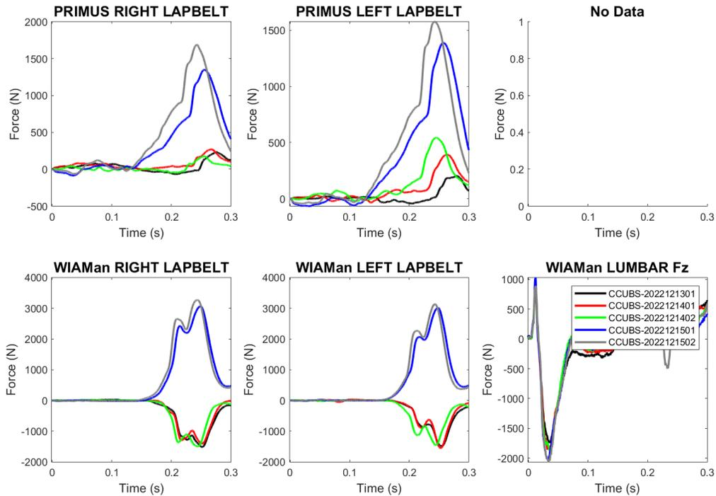
**Figure 6 SAE Channel Class CFC60 Lapbelt Loads and CFC600 HIII Lumbar Vertical Load (150g)**
