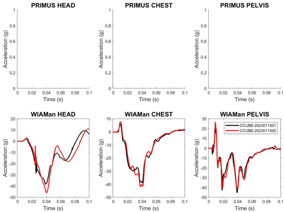
**Figure 11 SAE Channel Class CFC1000 Head, Chest, and Pelvic Accelerations (250g)**
