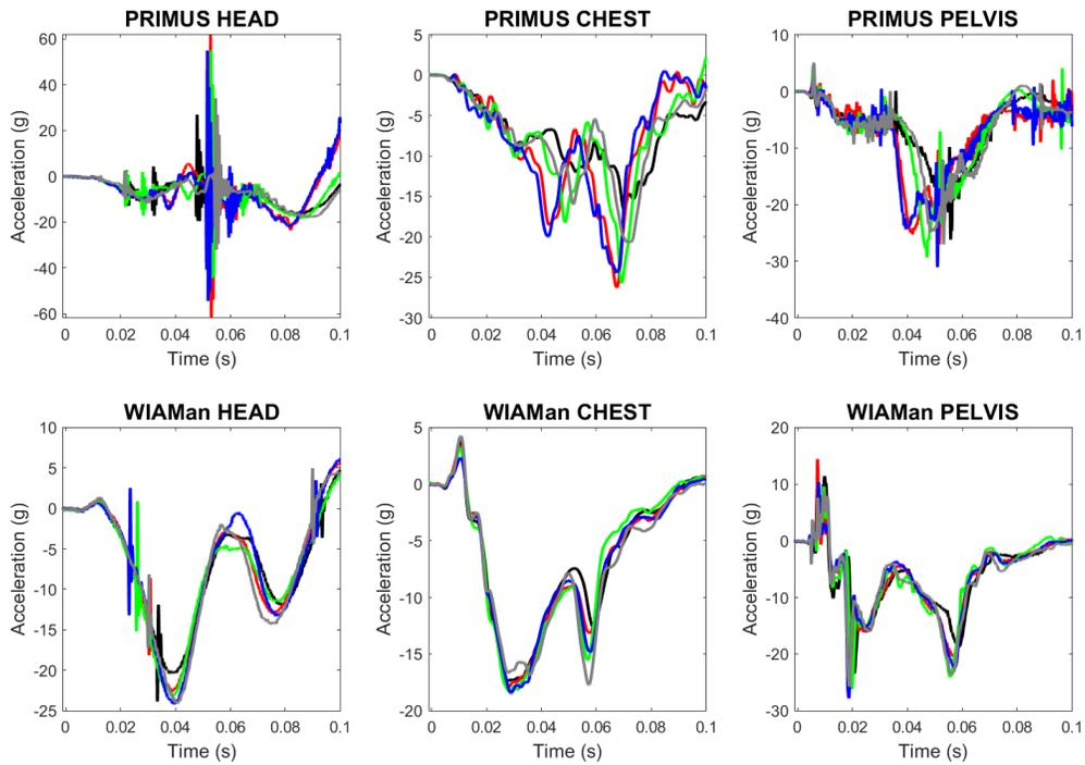
**Figure 10 SAE Channel Class CFC1000 Head, Chest, and Pelvic Accelerations (150g)**
