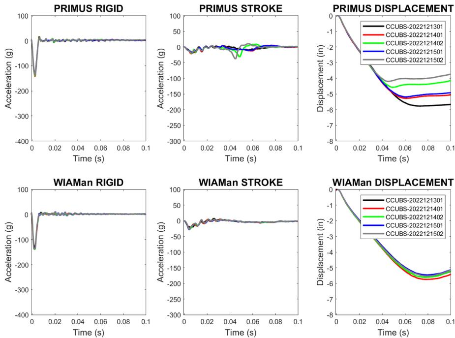
**Figure 3 SAE Channel Class CFC180 Seat Accelerations and Vertical Displacement (150g)**
