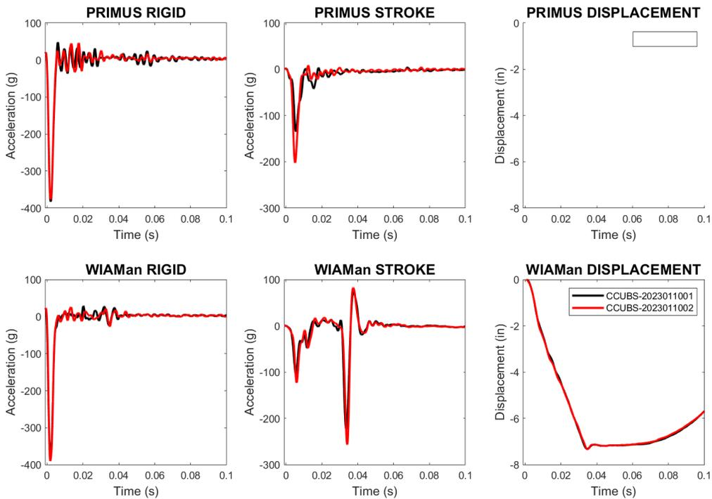
**Figure 5 SAE Channel Class CFC180 Seat Accelerations and Vertical Displacement (350g)**
