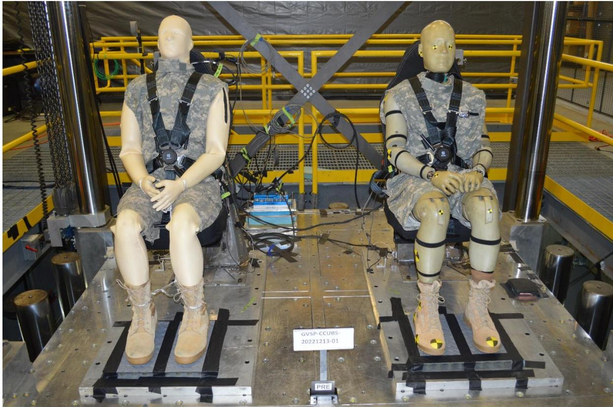
**Figure 1 CCUBS Test Setup. PRIMUS on the left (Position 2), WIAMAN on the right (Position 1).**
