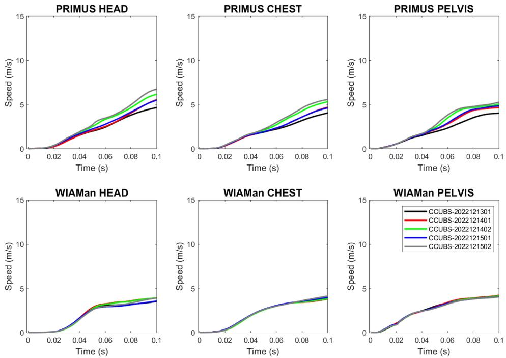
**Figure 14 Dummy Body Segment Speeds speeds(150g)**
