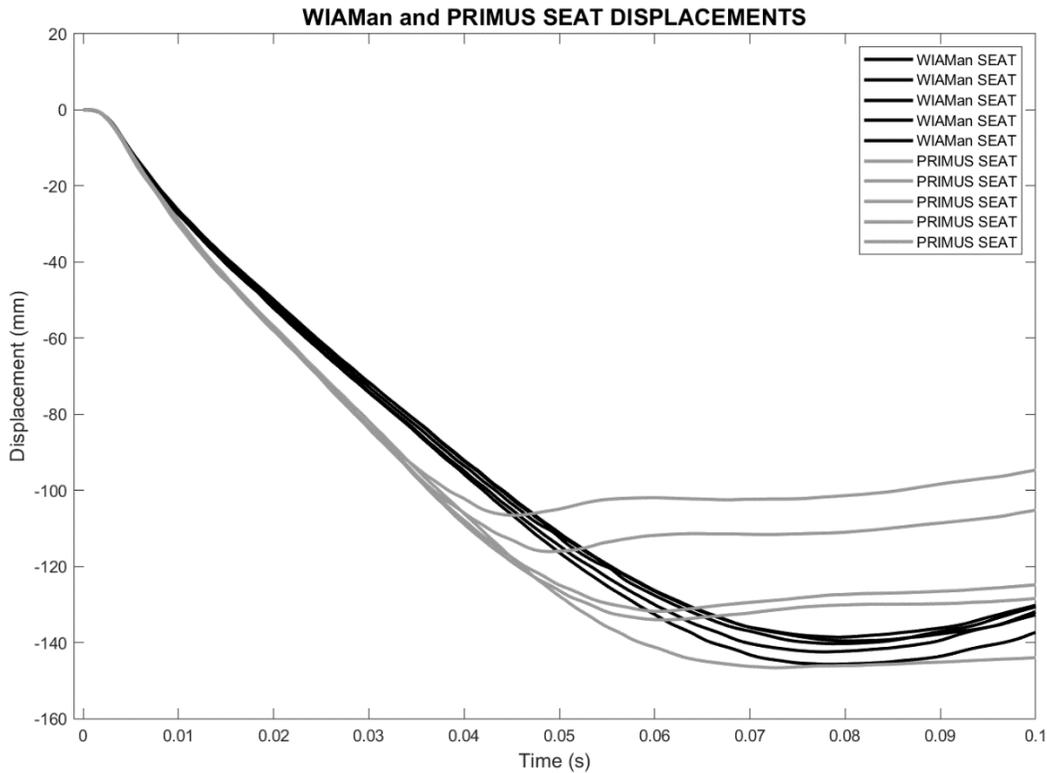
**Figure 17 Comparisons of Seat Displacement (WIAMan/PRIMUS) from 150g tests**
