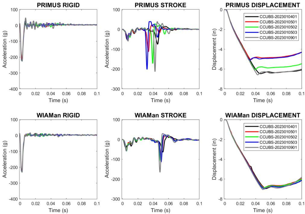
**Figure 4 SAE Channel Class CFC180 Seat Accelerations and Vertical Displacement (250g)**
