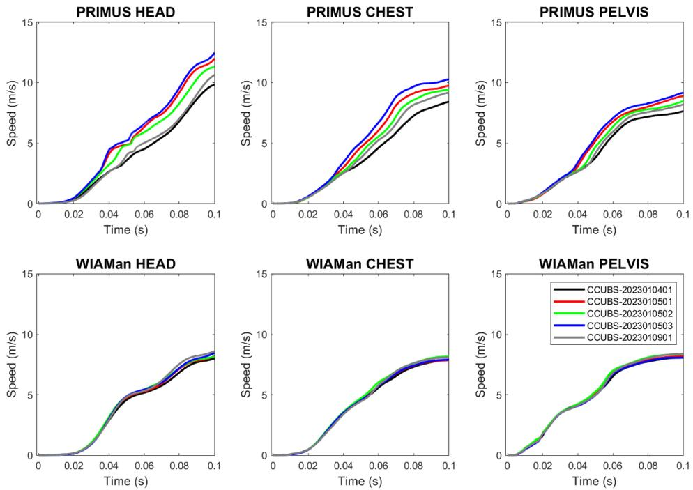
**Figure 15 Dummy Body Segment Speeds speeds(250g)**
