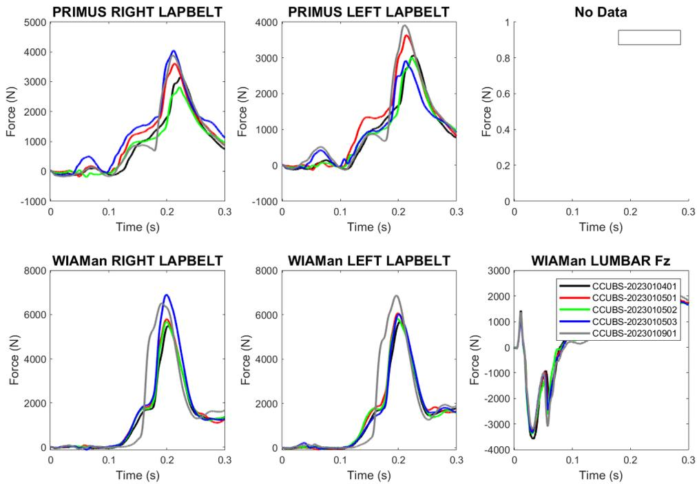
Figure 7 SAE Channel Class CFC60 Lapbelt Loads and CFC600 HIII Lumbar Vertical Load (250g)
